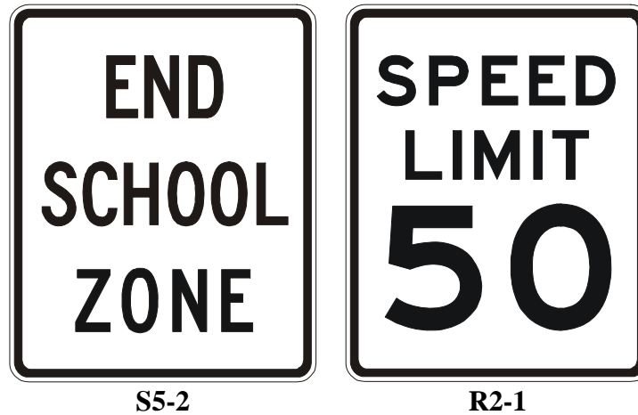
Figure 3-3. Examples of End of School Zone Signs.
