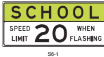
Figure 3-2. Example of School Speed Limit Assembly for Over Roadway.
