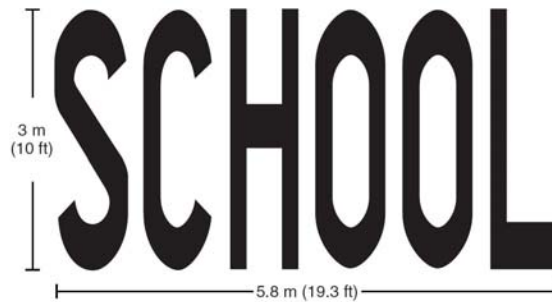
Figure 3-4. Examples of SCHOOL markings.
